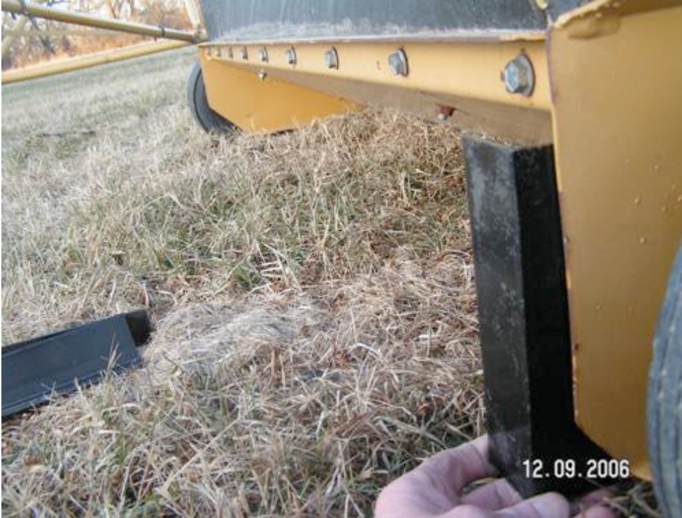
Inside mounting of angle iron bracket-- pushed out ward about 1/2"
