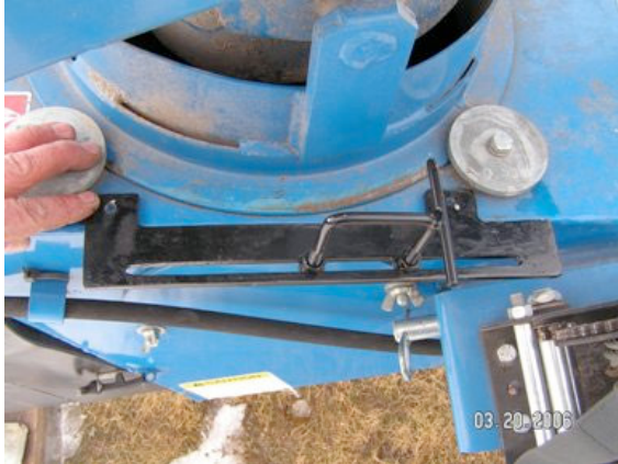
Picture showing proper position of side bracket on the 10" auger.
