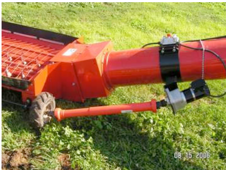
Complete motor and driveshaft and shield installed
