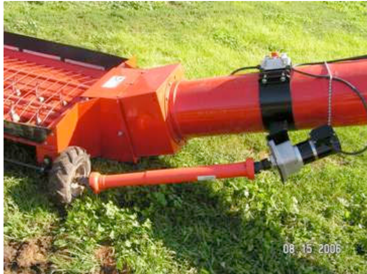
Complete motor and driveshaft and shield installed
