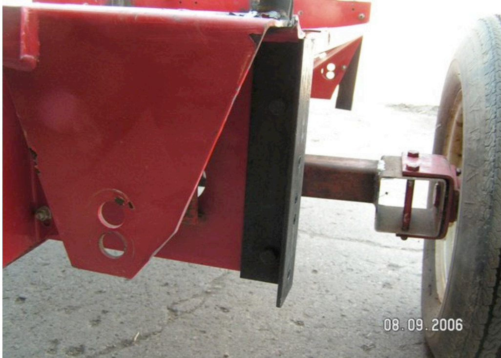
Similar picture showing the outside 7" angle iron mounted to hopper with 2 3/8"x 1" bolts and nuts.
