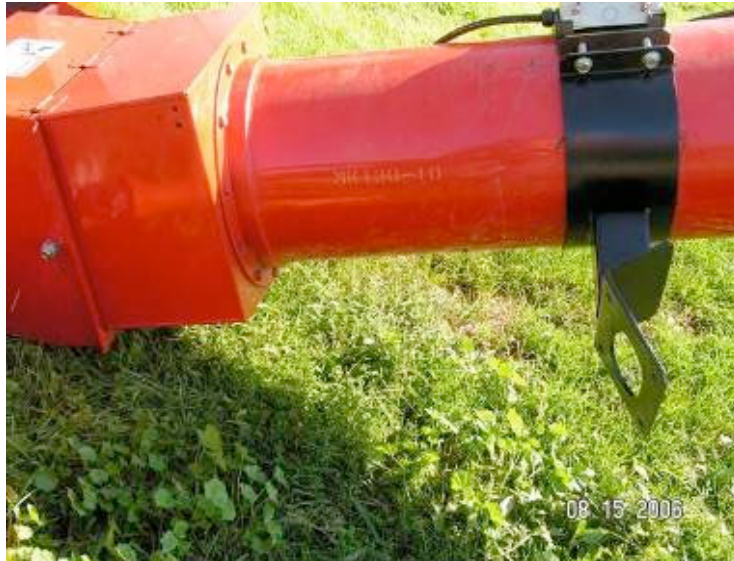
Picture showing proper mounting of motor mount - 15- 20" from intake of hopper
