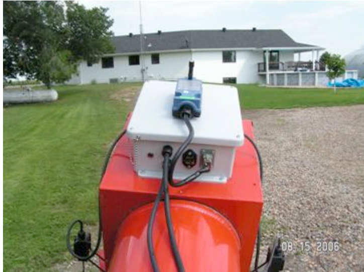
Picture showing control box mounted on swing hopper head.
