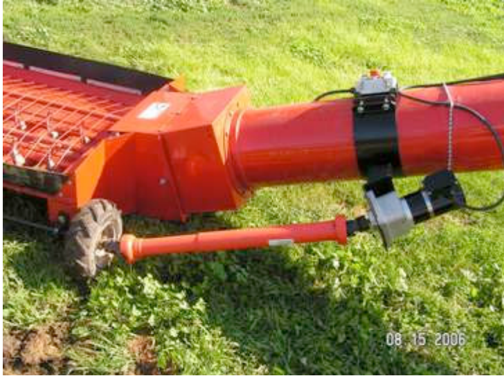
Complete motor and driveshaft and shield installed
