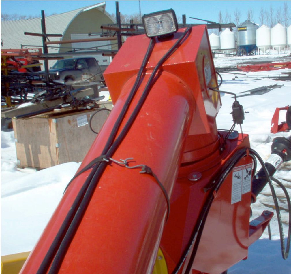
Position of work light and cables. Make sure cables are securely fastened.
