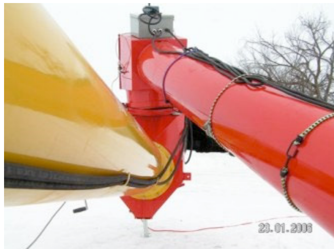
Swing hopper tube with 6" of clearance between main auger tube.
