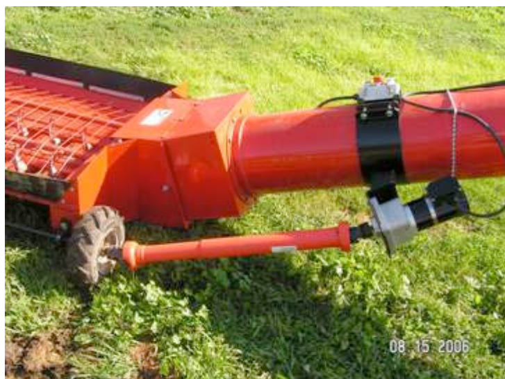
Complete motor and driveshaft and shield installed
