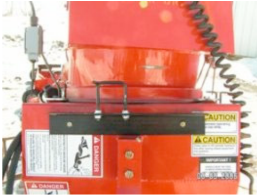
Placement of front bracket on 13" Westfield or the 10" Mayrath & Hutchinson
