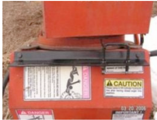
Placement of front bracket on 10" Westfield or the 13" Mayrath & Hutchinson
