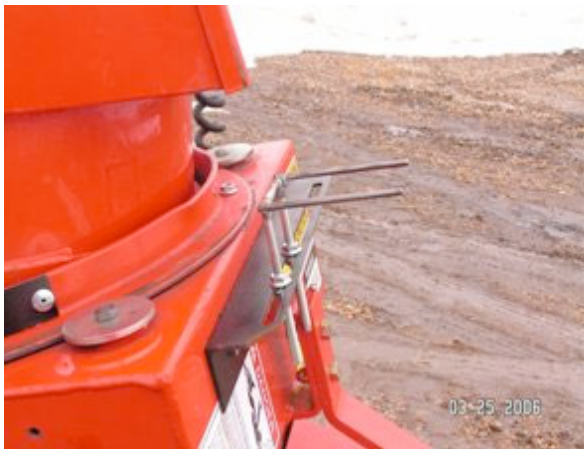
Placement of front bracket on 13" Westfield or the 10" Mayrath & Hutchinson
