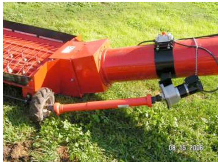
Complete motor and driveshaft and shield installed
