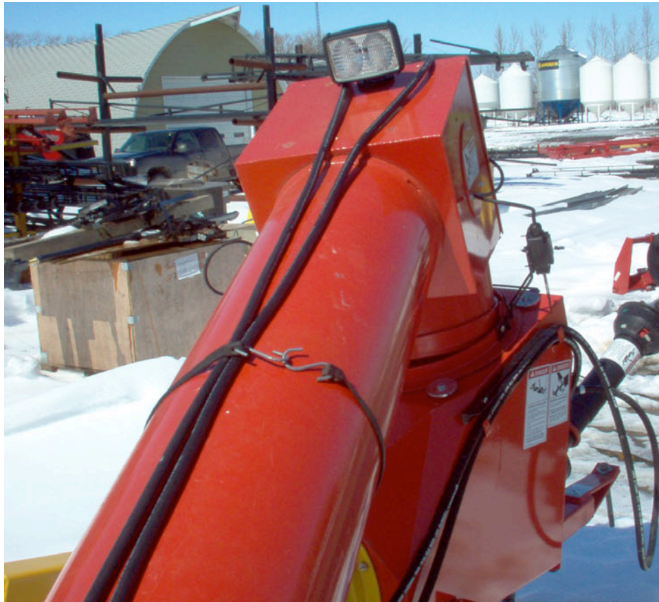
Position of work light and cables. Make sure cables are securely fastened.
