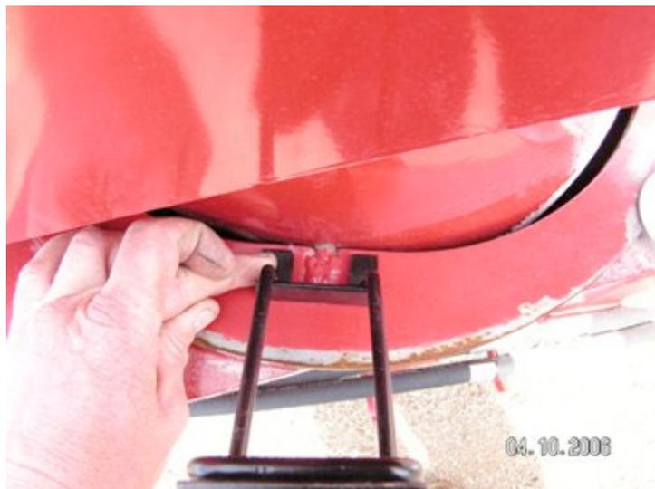
Picture showing position of location placement of holder on pivot ring. Leave 1/16" to 1/8" clearance between holder and tube of auger. Moving mounting out farther than 1/8" could make holder come in contact with factory hold down washers when swing hopper swings to the left or right.
