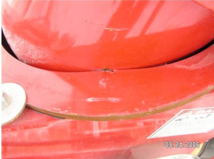
Picture showing where the limit switch holders will be placed on pivot ring. The holder will be centered over the factory pin that is used to pivot the swing tube on the pivot ring.
