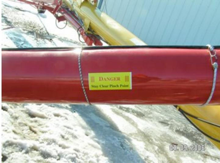
Install one each on both sides of swing tube centered from top to bottom
