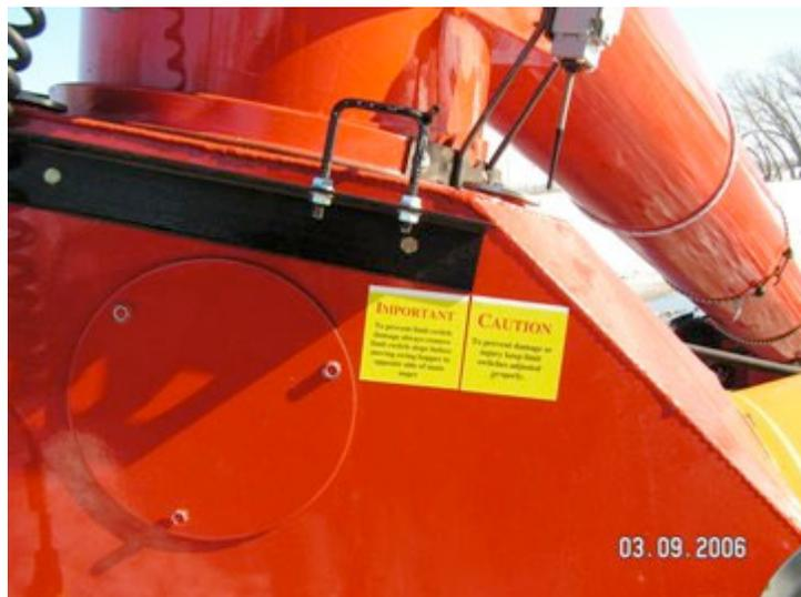
Place one each on both sides of the auger boot
