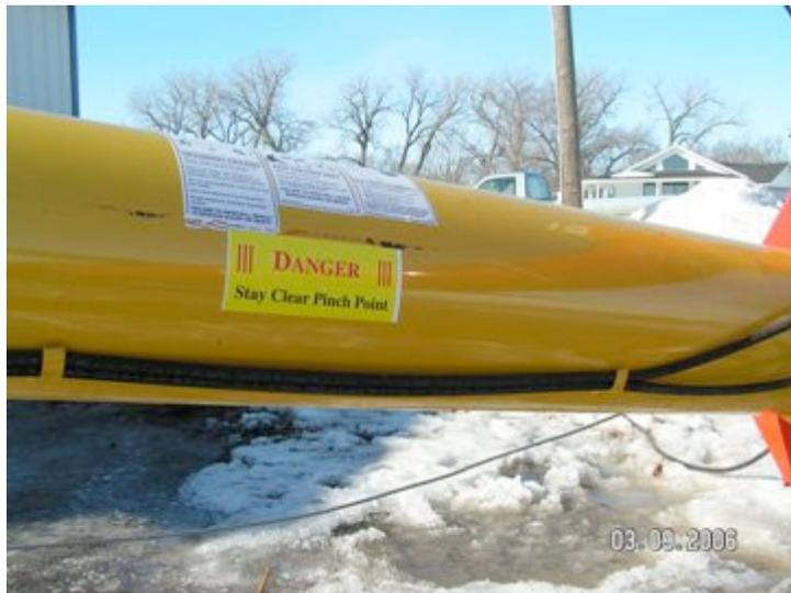
Install one each on both sides of main auger tube approximately 3-4 feet from the beginning of the tube.
