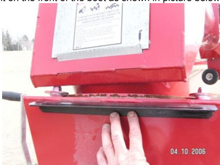
Picture showing proper placement of front mounting bracket parallel with auger boot and lowered approximately  $\frac{1}{4}$ " below welding.
