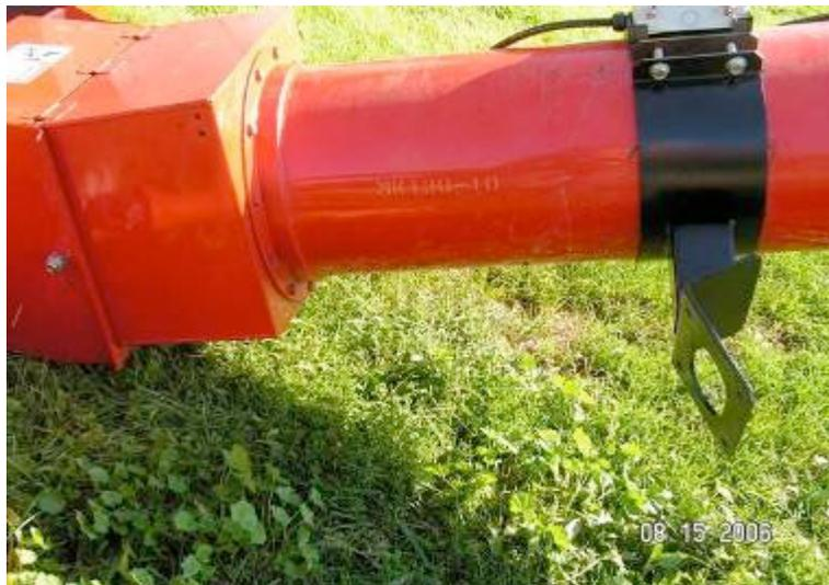
Proper mounting of motor mount-- 15-20" from intake of hopper
