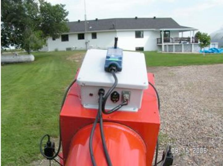
Similar picture showing control box mounted on top of swing auger head.
