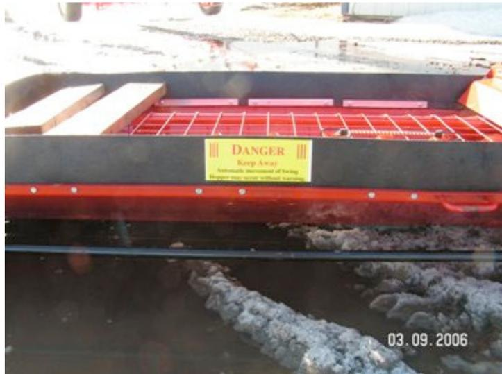
Install one on each side and end of the swing hopper
