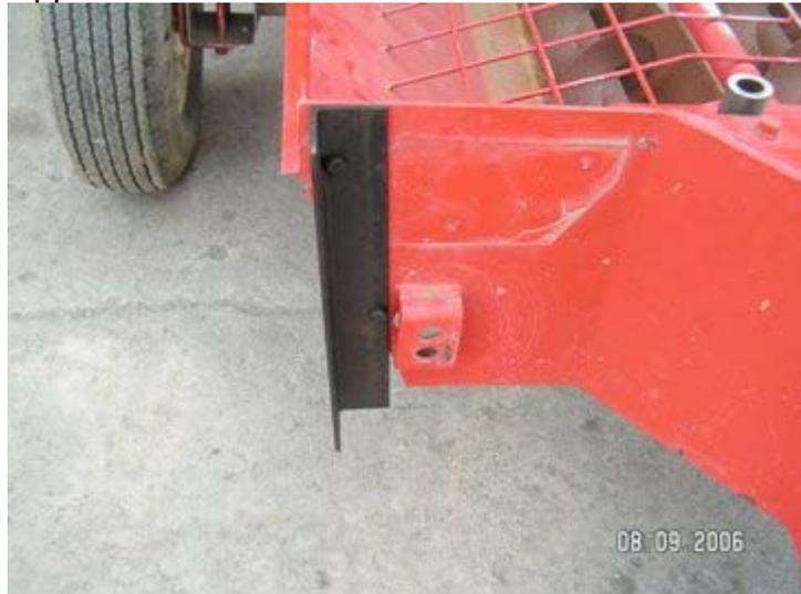
Picture showing 13" angle iron bolted with 2 3/8"x1" bolts and nuts. Angle iron is flush with top of hopper.
