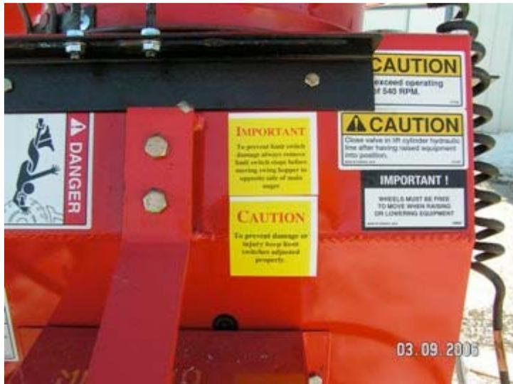
Place one each--important prevent limit switch damage
