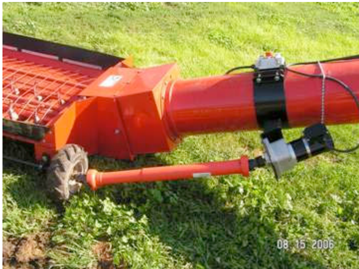
Complete motor and driveshaft and shield installed
