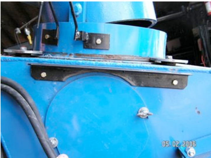
Similar picture showing proper position of side bracket on 13" auger 6" from front of boot.
