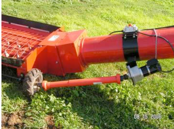
Complete motor, driveshaft and shield installed
